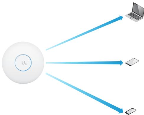
MU-MIMO with 2x2 and 1x1 clients: The UniFi SHD AP communicates with one 2x2 client and two 1x1 clients at a time.
