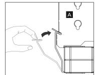
Attach the fan using the supplied steel clips for maximum cooling performance
