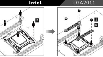
For LGA2011, screw the "Screw F" on the motherboard directly without the "Backplate C"
