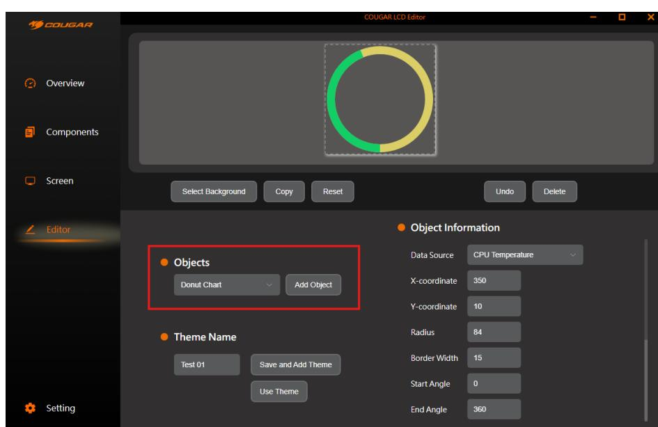
2. In the Object Information section, you can further configure properties such as data type, position, font, and color.
