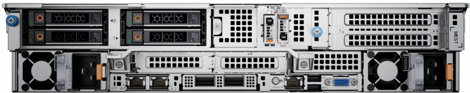
Figure 11. Rear view of the system with 4 x 2.5-inch rear drive module
