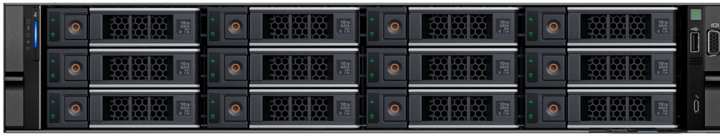
Figure 4. Front view of 12 x 3.5-inch drive system
